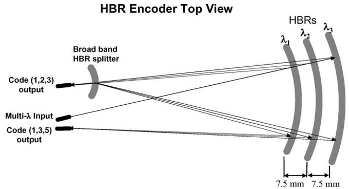
Fig. 7. Schematic top view of the  $1 \times 2$  integrated holographic OCDMA encoder. The optical path for generation of code (1, 2, 3) is shown. A broadband HBR splits off a fraction of the exiting (1, 2, 3) code sequence and converts it to code (1, 3, 5) by double passing of the HBR array. Dimensions in the figure are not to scale.
