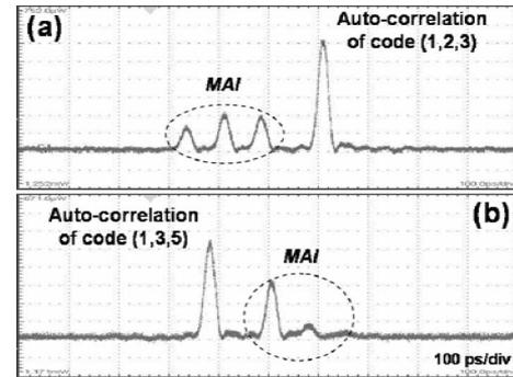
Fig. 9. The decoded autocorrelation peaks for (a) code (1, 2, 3) and (b) code (1, 3, 5) and cross-correlation signals arising from the nonmatching input.
