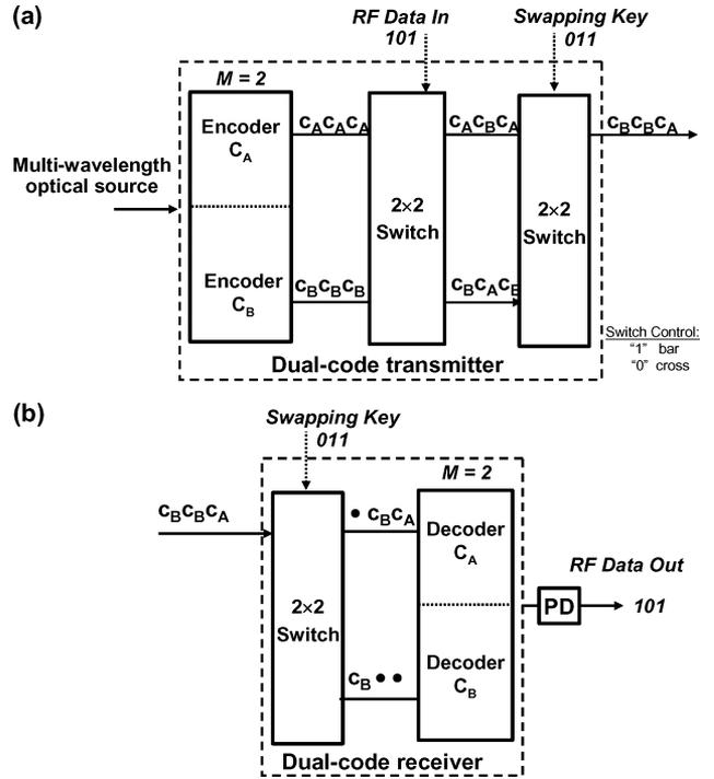
Fig. 13. Schematic of (a) dual-code transmitter and (b) receiver.
