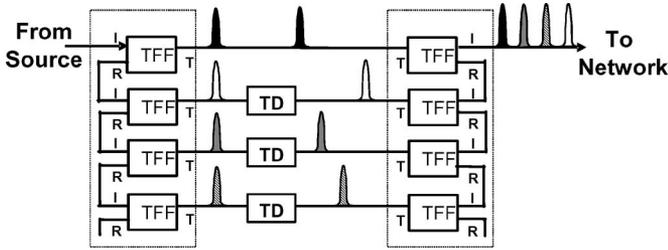
Fig. 3. Schematic of a WHTS encoder with four wavelengths in the code and using TFFs (I: input port; T: transmitted port; R: reflected port) technologies.
