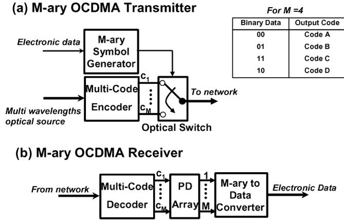
Fig. 12. Implementation of M-ary OCDMA (a) transmitter and (b) receiver.
