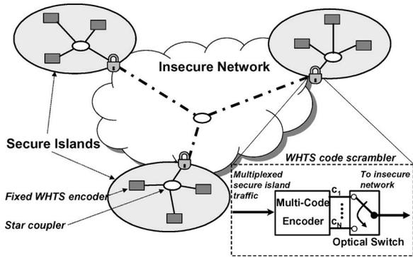
Fig. 10. Schematic of a shared code scrambling network. Nodes are represented by the shaded rectangles and the lock represents the shared code scrambler. The inset shows the architecture of the WHTS code scrambler.
