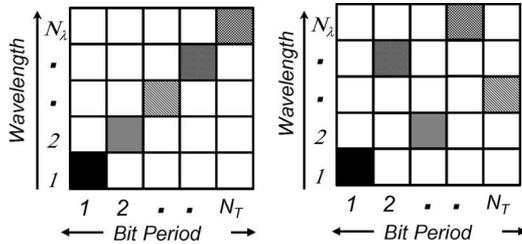
Fig. 1. Two code sequences for WHTS OCDMA. The bit period is divided into  $N_T$  chips ( $N_T$ : code length), and code sequences are formed by placing  $w$  ( $w$ : code weight) pulses of different wavelengths ( $N_\lambda$ : number of different wavelengths) in them.
