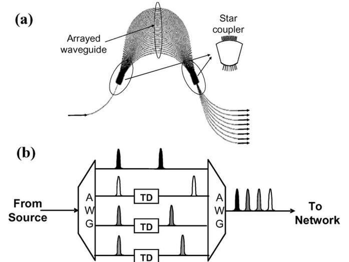
Fig. 5. Schematic of (a) an AWG [34] and (b) a WHTS encoder with four wavelengths in the code using AWG technologies.
