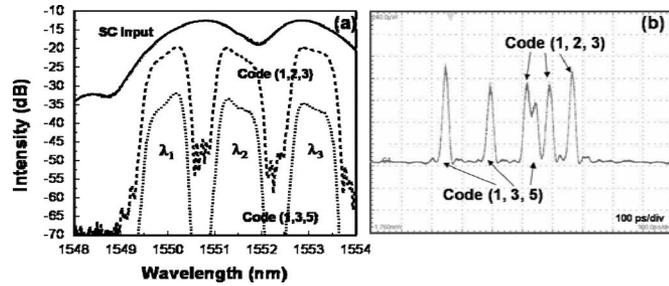
Fig. 8. (a) Spectra and (b) time signatures of the generated WHTS codes.
