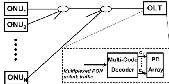
Fig. 11. Schematic of a WHTS OCDMA PON uplink with a multicode decoder configuration at OLT.
