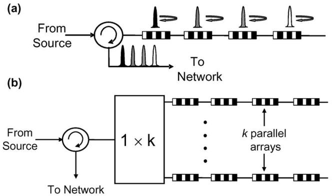
Fig. 4. (a) Schematic of a WHTS encoder with four wavelengths in the code and using a linear array of FBG. (b) Parallel linear array of FBGs allows implementation of MPPC codes.  $k$  is the maximum number of wavelengths in the same column of the code matrix [32].
