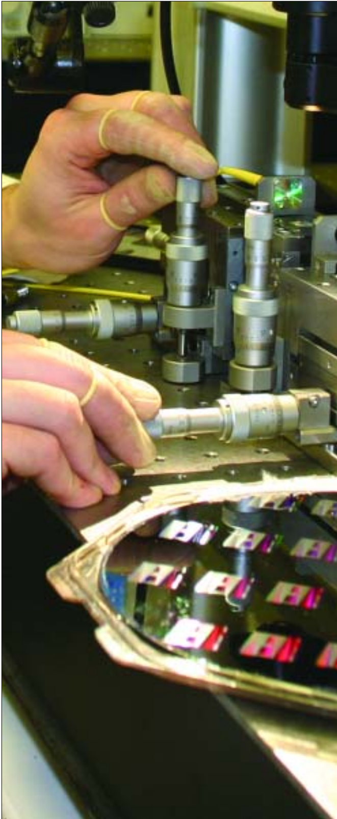
Testing planar waveguide holographic Bragg reflectors. ( Foreground ) Eight-inch silica-on-silicon wafer inscribed with stepped HBR test structures. The wafer shown has no upper silica cladding. ( Background ) Mounted HBR die under examination.
